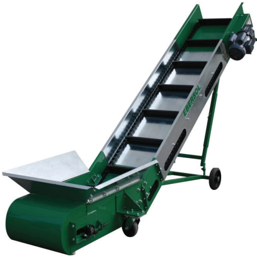
Industrial Conveyors and feed hoppers
